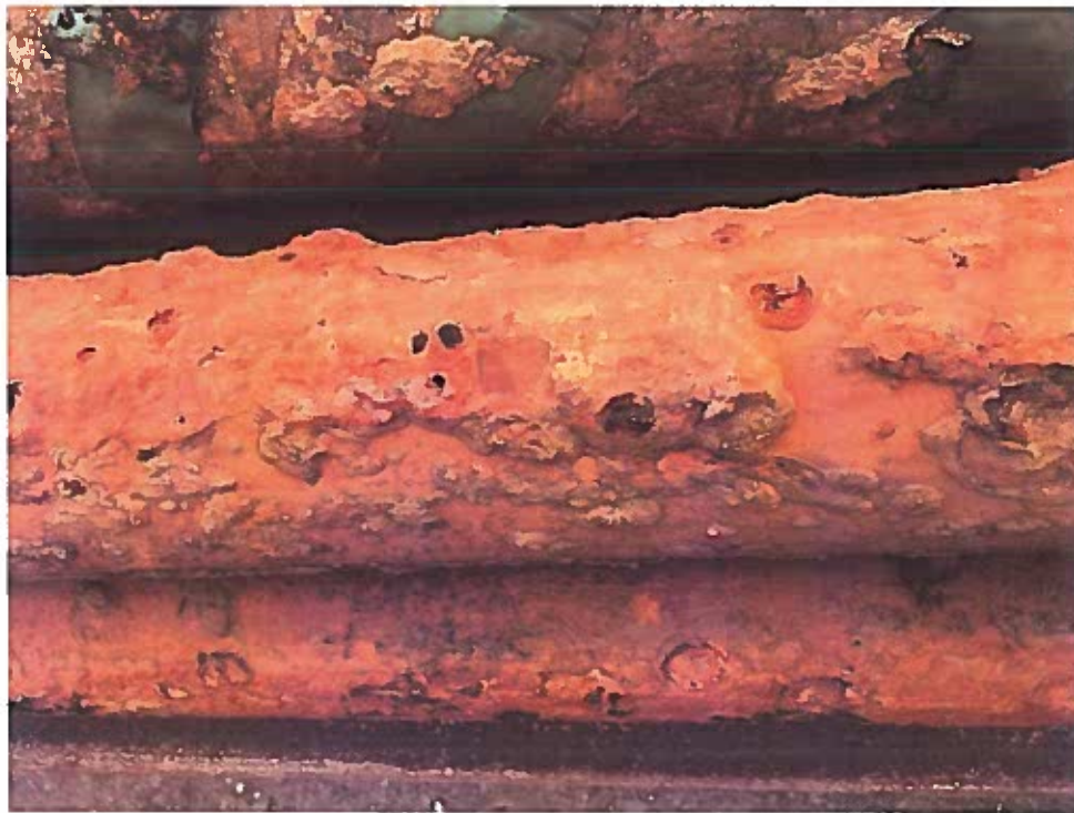
DETERIORATED WELL DROP-PIPE THAT SUPPORTS THE PUMP & MOTOR
