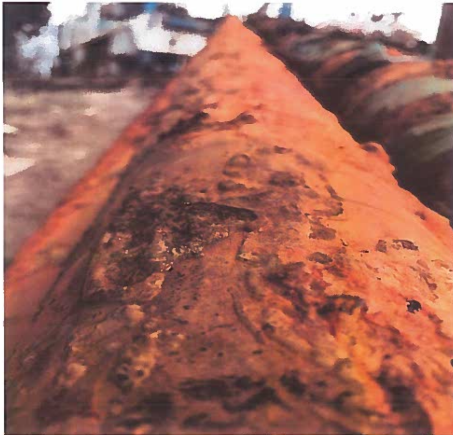
DETERIORATED WELL DROP-PIPE THAT SUPPORTS THE PUMP & MOTOR
