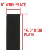
3/8" THICK WELDED ALUMINUM **MOUNTING PLATE** WITH .50 HOLES TO ACCOMMODATE 3/8" GALVANIZED THREADED ROO
