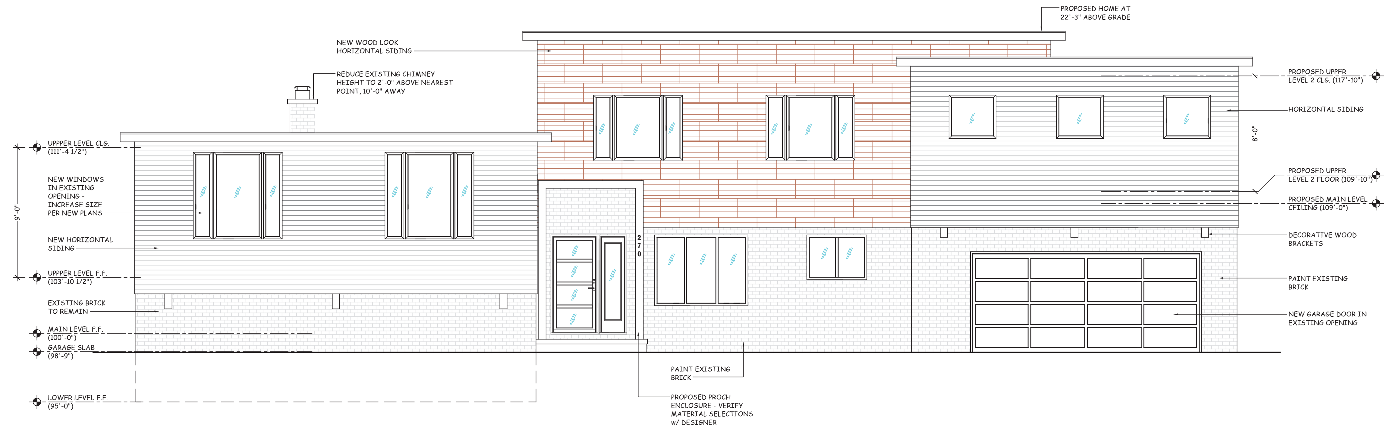
PROPOSED FRONT ELEVATION 'E' SCALE: 1/4" = 1'-0"
