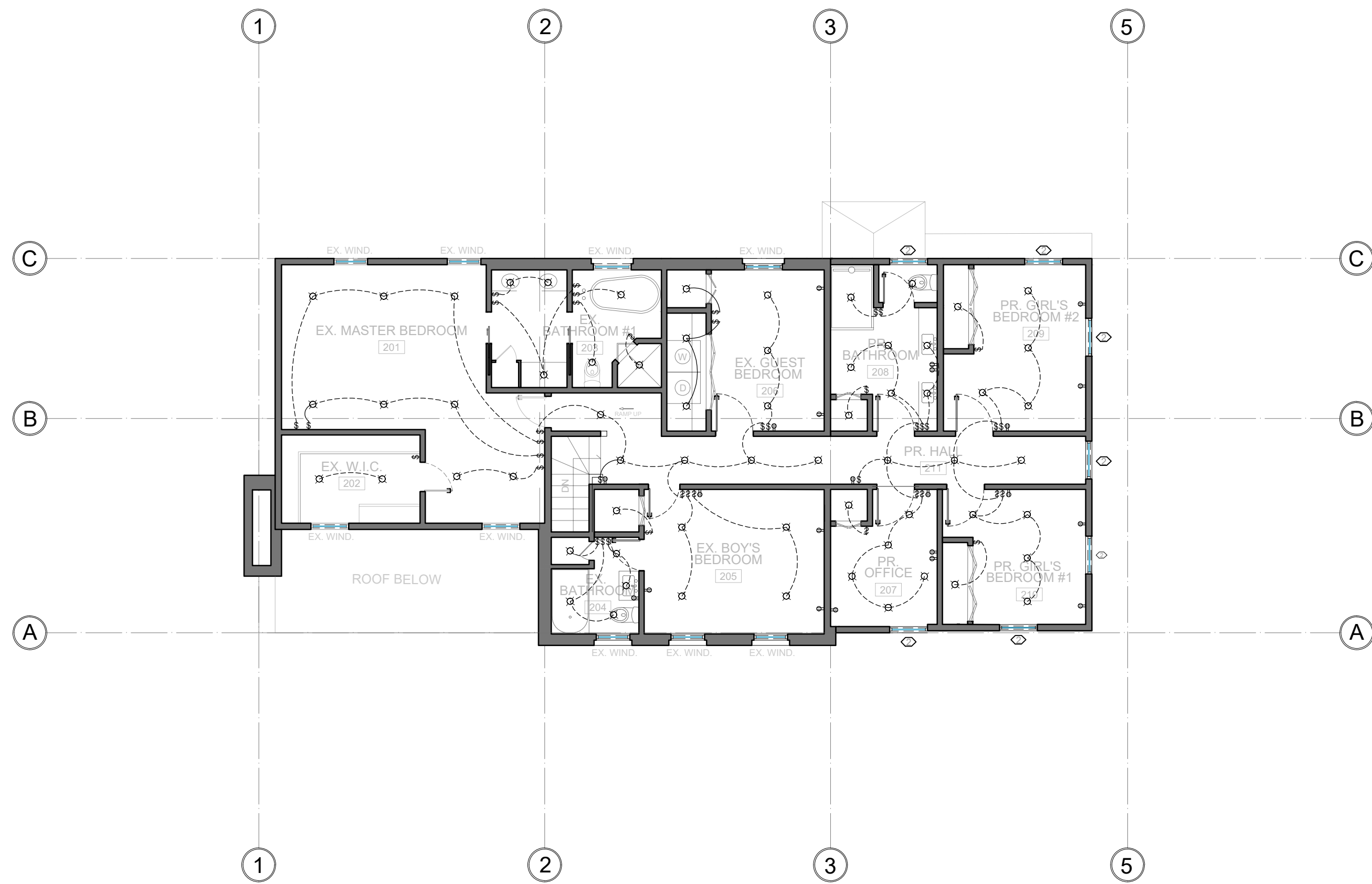
SECOND FLOOR LIGHTING PLAN SCALE 1/8"=1'-0"
