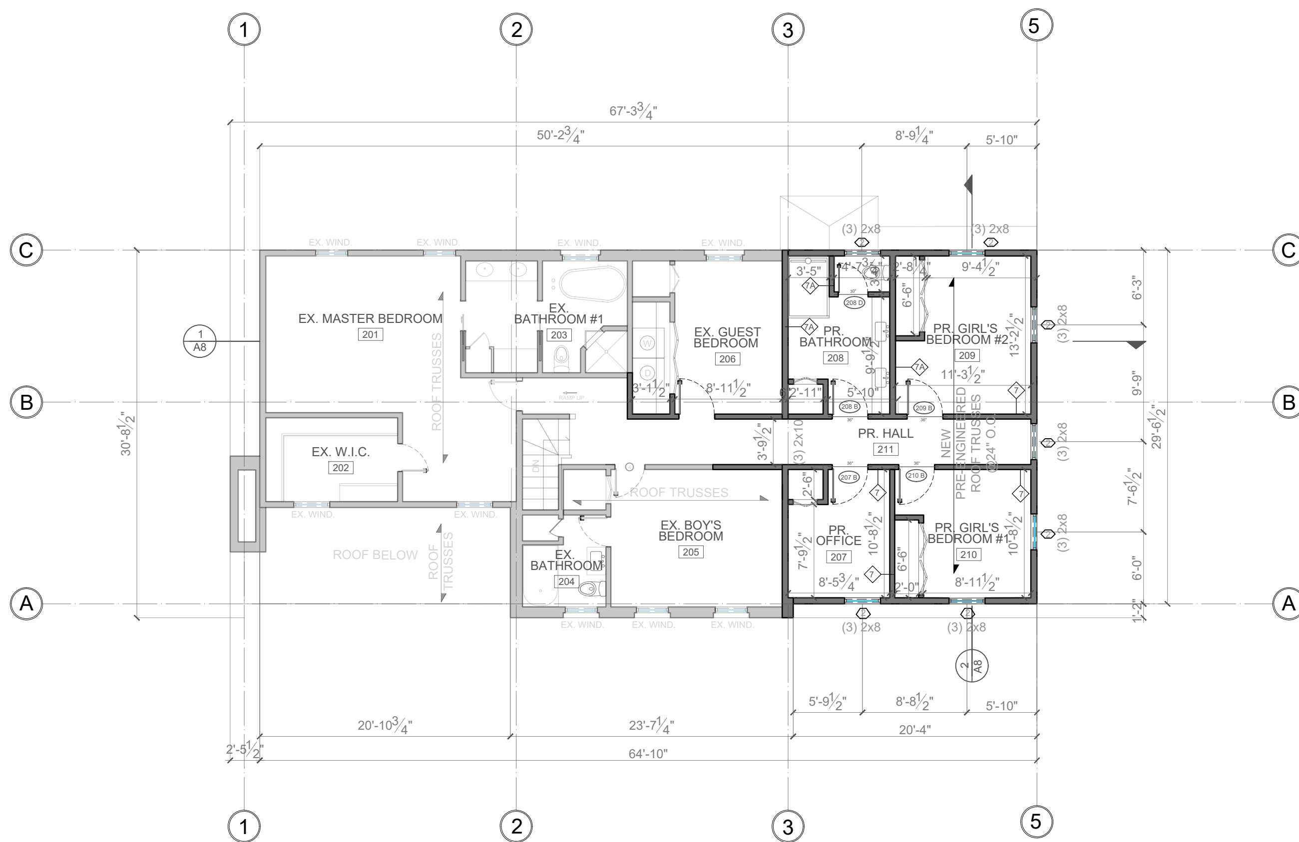
PROPOSED SECOND FLOOR PLAN SCALE 1/8"=1'-0"
