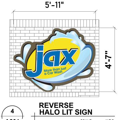
SIGN CALCULATIONS (WOODWARD AVE. FACADE / EAST ELEVATION) 28" REVERSE HALO LIT CHANNEL LETTERS READING 'KAR WASH' = **33 SF** (PROPOSED) (1) REVERSE HALO LIT SIGN = 27.1 SF (PROPOSED) TOTAL SQUARE FOOTAGE OF PROPOSED SIGNAGE = **60.1 SF** (TOTAL)
