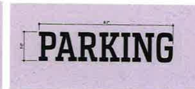
MATERIAL: ALUMINUM FINISH: BLACK POWDER COA MOUNTING: FLUSH MOUNT LETTER DEPTH: 8"
