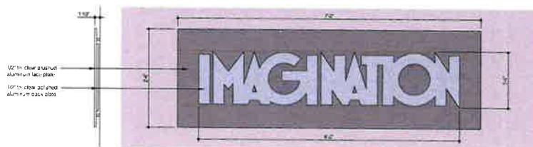
MATERIAL: ALUMINUM FINISH: CLEAR POLISHED LETTERING CLEAR BRUSHED SURROUND MOUNTING: FLUSH MOUNT DEPTH: 1 1/2"
