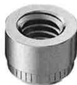
18-8 Stainless Steel Press-Fit Nut for Sheet Metal (3/8"-16 Thread Size, for 0.125" Minimum Panel Thickness)
