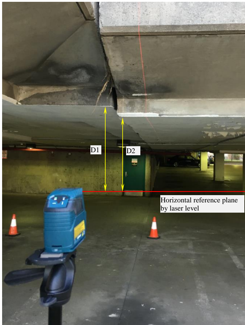
Figure 5. Slab differential deflection measurement
