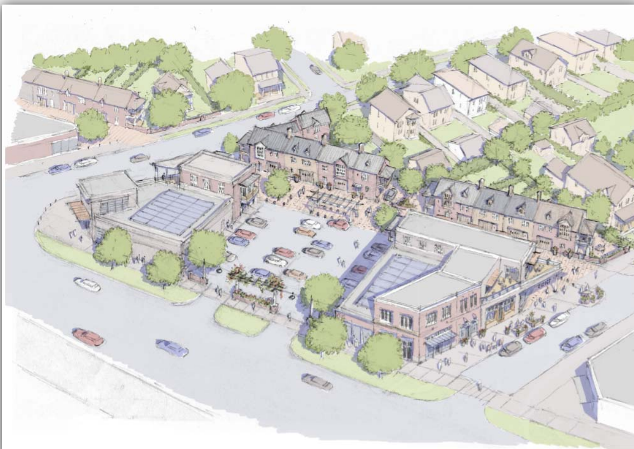
Figure C.6-13. Neighborhood Sleeve block configuration which consolidates parking mid-block and creates small neighborhood-focused nodes along the east-west streets.
