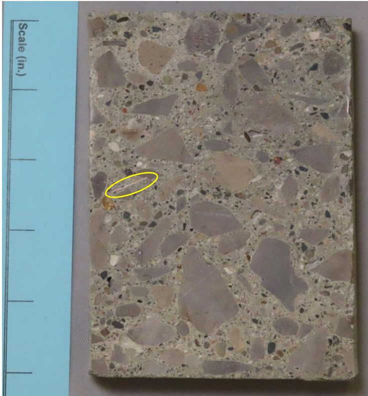
Figure 2. Lapped surface of Core 2. Residual copper left from a paste scratch hardness test is circled on the image.
