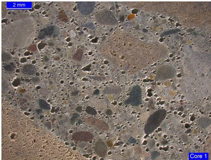
Figure 7. Air void system in Core 1. Entrained air voids appear primarily as small, black circular areas due to the use of low-angle light illumination.
