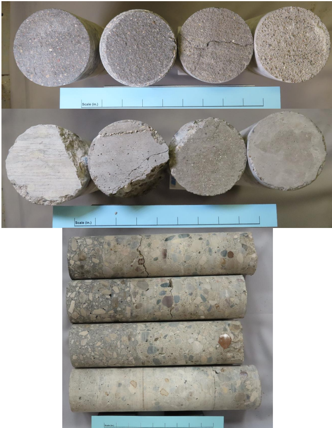
Figure 1. The as-received appearance of the tops (upper), bottoms (middle), and sides (lower) of Cores 1 through 4 are pictured. In the upper and middle images, cores are pictured from left to right, and in the lower image, cores are pictured from top to bottom.
