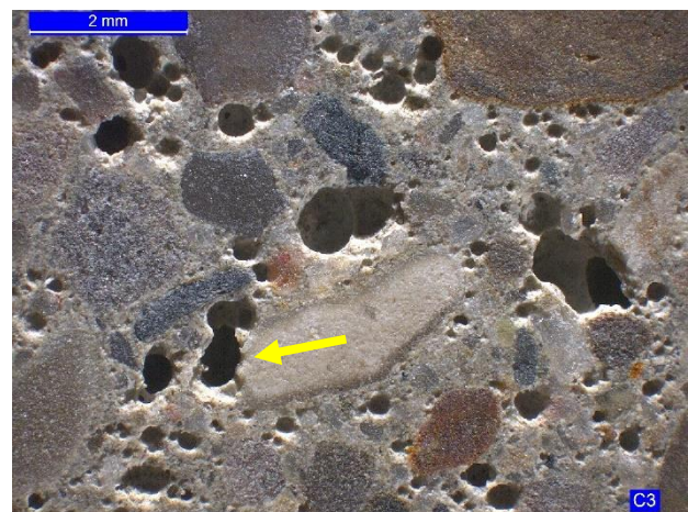
Figure 3. Darkened rims (arrows) are pictured around several chert particles within Core 3. The rim is discontinuous adjacent the air void in the right image, suggesting its formation after being incorporated into the concrete, such as from ASR. No distress was associated with any of these particles.
