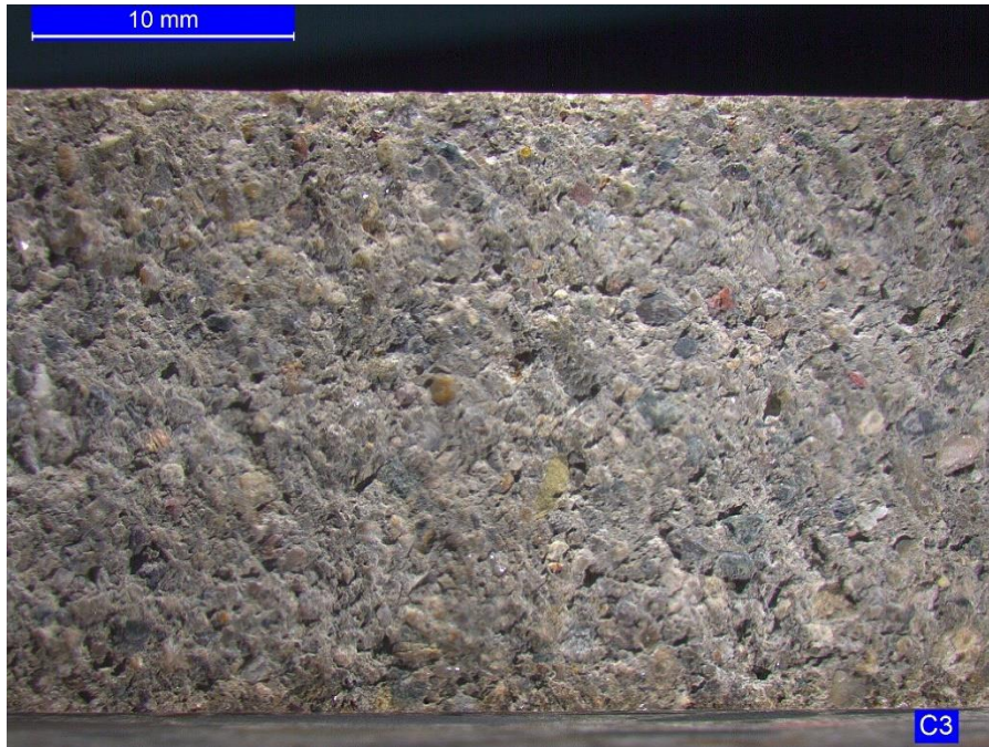
Figure 6. The top eroded surface of Core 3 with partially exposed fine aggregates.
