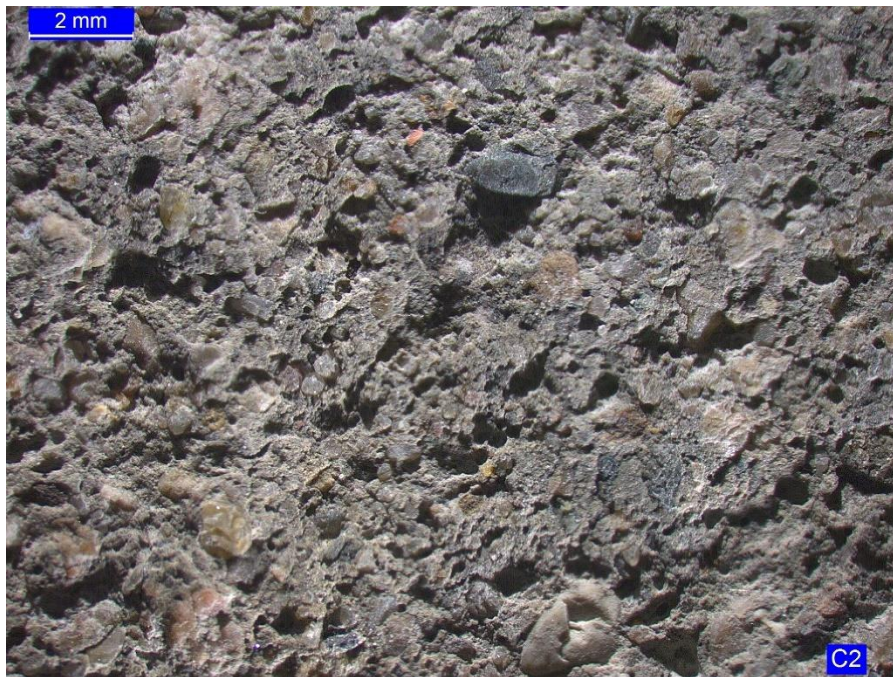
Figure 7. Thin, elongate voids on the top surface of Core 2.
