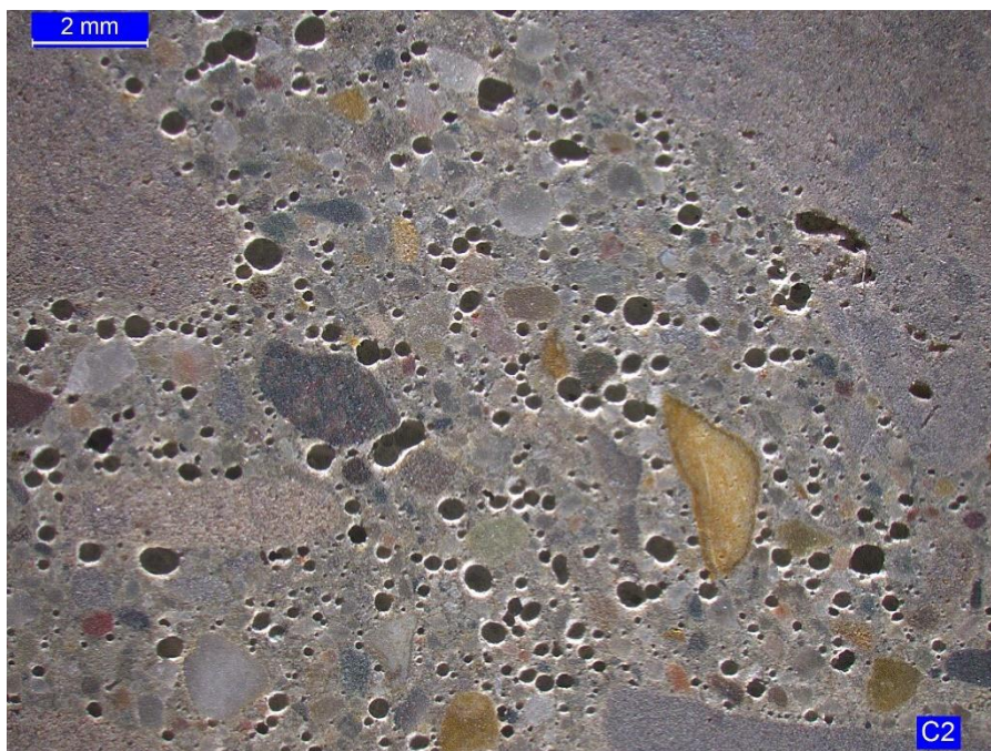
Figure 5. Air void system in Core 2. Entrained air voids appear primarily as small, black circular areas due to the use of low-angle light illumination.
