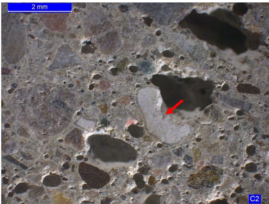
Figure 3. A chert fine aggregate contains a discontinuous reaction rim adjacent the void (arrow).
