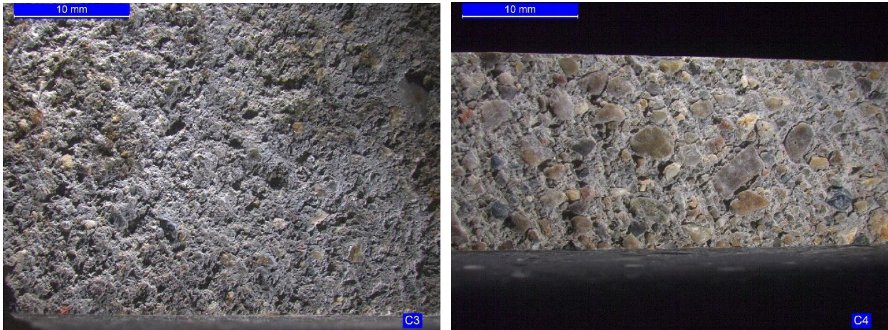
Figure 9. The eroded top surfaces of the toppings in Core 3 (left) and Core 4 (right). A greater number of aggregates are exposed on the surface of Core 4. Note that the topping is compositionally dissimilar in Core 4 compared to Cores 1, 2, and 3.
