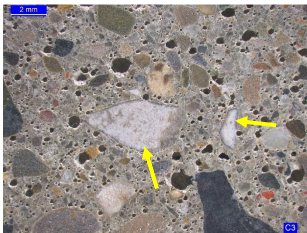
Figure 3. Darkened rims (arrows) are pictured around several chert particles within Core 3. The rim is discontinuous adjacent the air void in the right image, suggesting its formation after being incorporated into the concrete, such as from ASR. No distress was associated with any of these particles.
