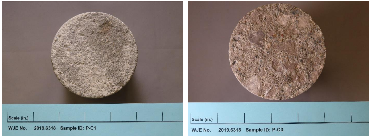
Figure 8. The eroded top surfaces of Core 1 (left) and Core 3 (right).
