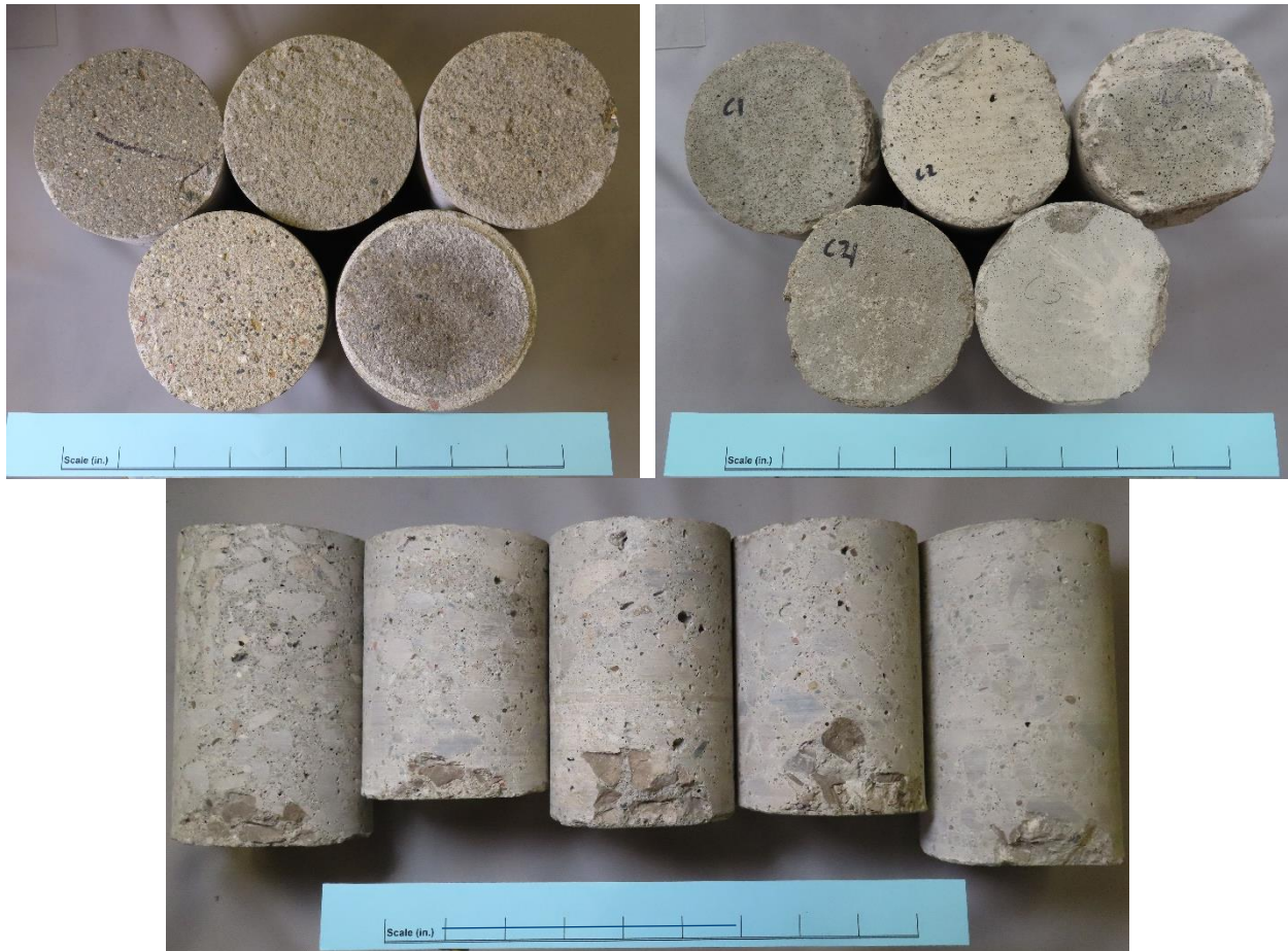
Figure 1. The as-received appearance of the tops (upper left), bottoms (upper right), and sides (lower) of Cores 1 through 5 are pictured. In the lower image, Cores 1 through 5 are pictured from the left to right, respectively.
