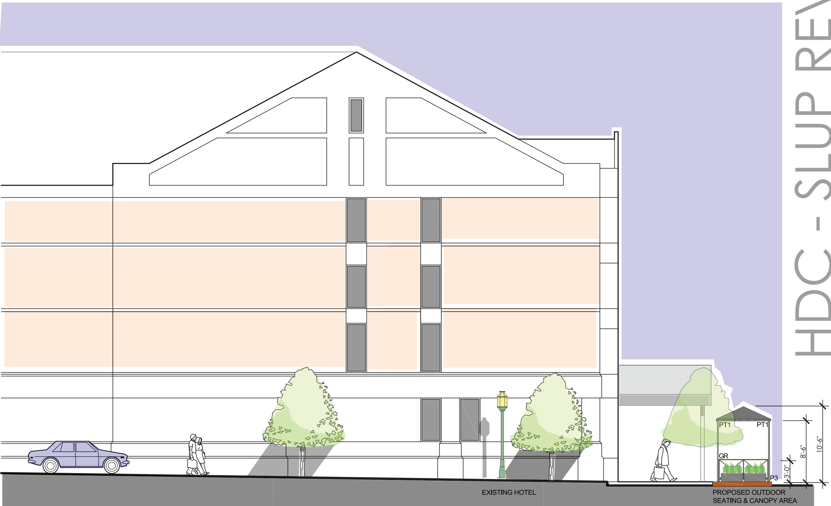
4 SD 1.03 Partial West Elevation Outdoor Dining 1/8" = 1'-0"
