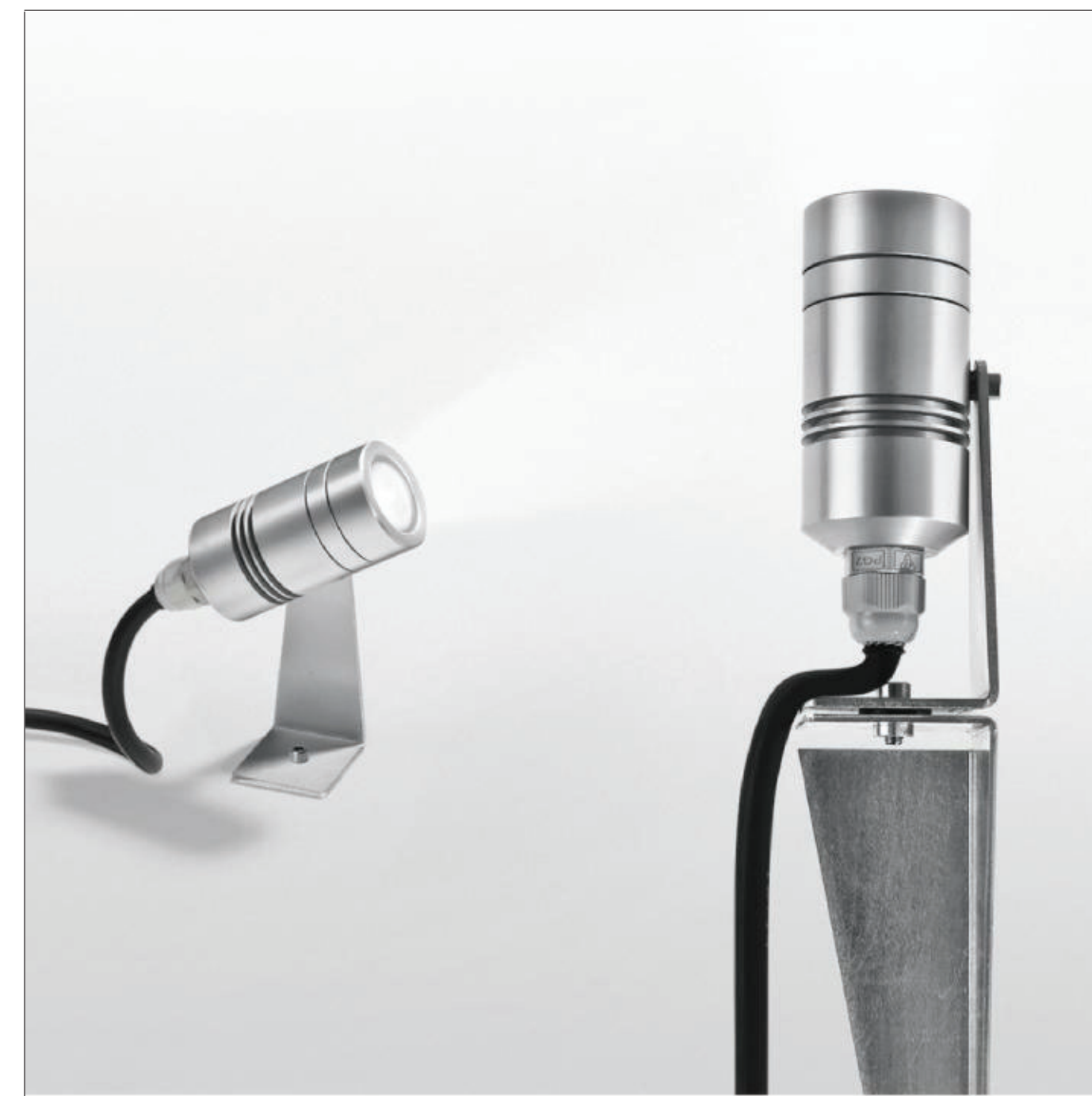
Artemide Mini Spot LED 2W > 80 CRI /17° beam spread Dim = 1 1/4" dia x 4" height 100 lm
