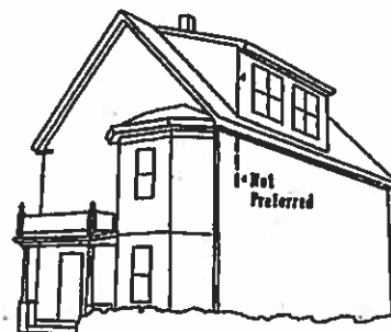
Figure 2: Setting the front wall of a dormer flush with the main wall underneath is not recommended. See Fig. 6 for the preferred 1 ft. 6 in. setback.
