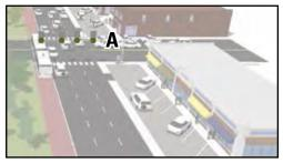
BRT vehicle proceeds through intersection on extended green light (A).
