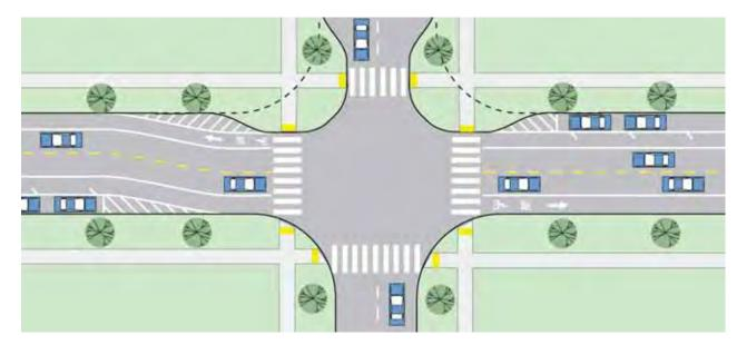
Pavement markings for the door swing zone are proposed between the on-street parking and the bike lane. See previous page for details.
