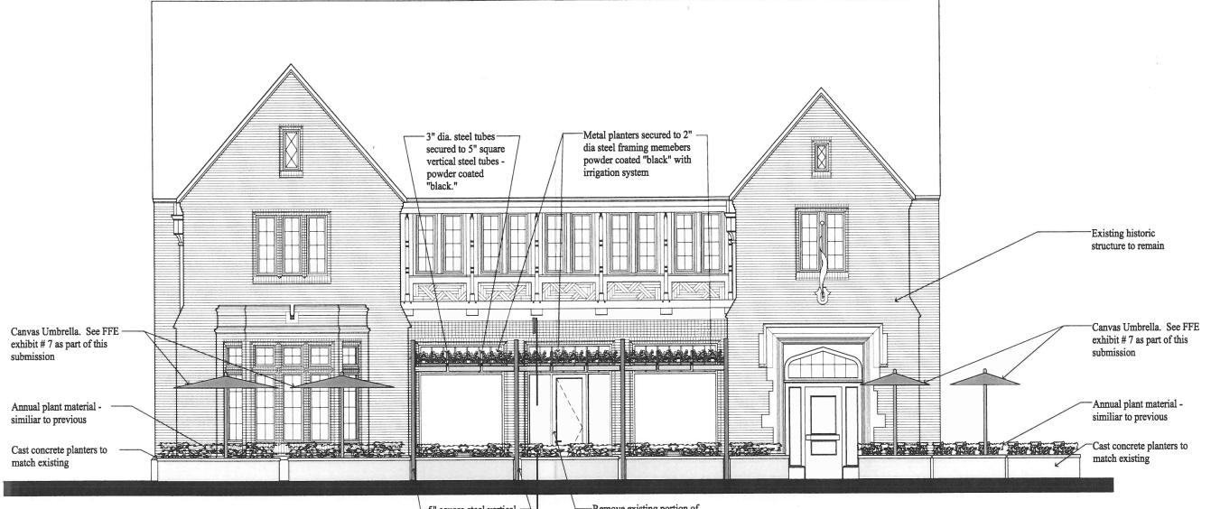
└─5" square steel vertical ─┘ tubes powder coated "black." Remove existing portion of glazing system and stone wainscot. Install new metal french door and sidelites with bronze finish to match existing.
