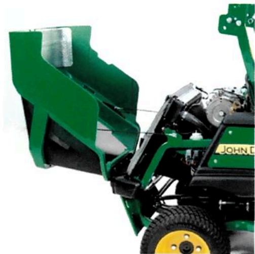
Hood open for access to engine
