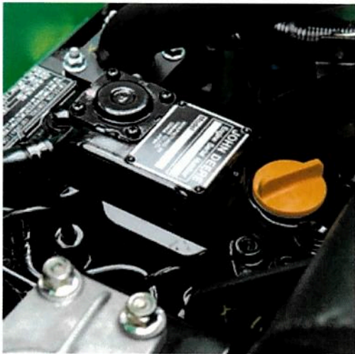
3-cylinder, liquid-cooled diesel engine
