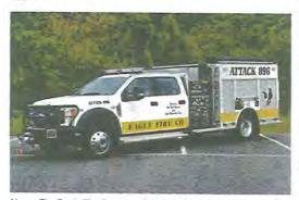
Above: The Eagle Fire Company Attack 896 KME Ford F-550 1,250gpm mini pumper. (Photos by KME.) Below: The rear of the unit with large roll-up compartment and hosebed.
