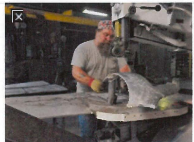
Removing vents and gates.
