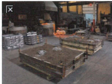
The sand mold ready for casting.
