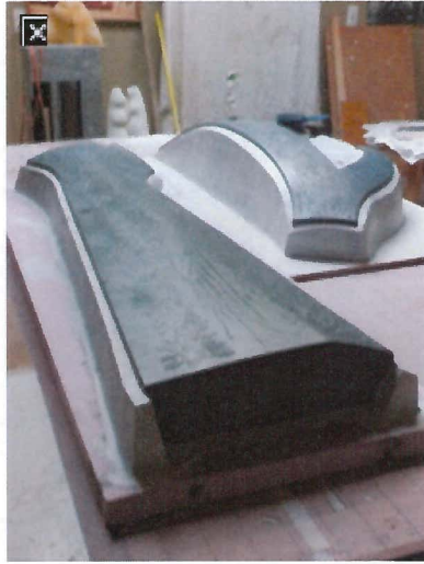
Plaster patterns on follow boards.
