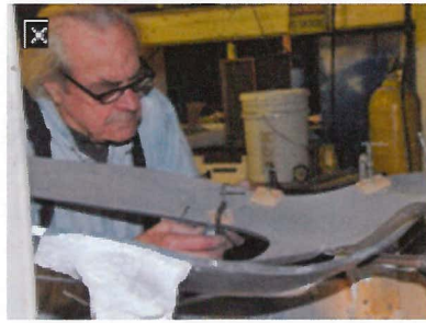
Clamping sections in position for welding.
