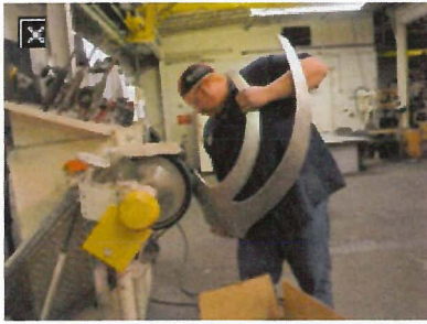
Grinding the joint before placing section on the jig.
