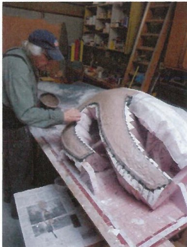
Plaster being applied to the styrofoam.
