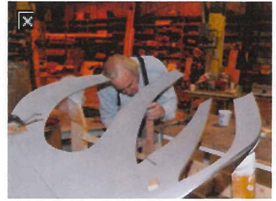
Cast aluminum section being adjusted on jig.
