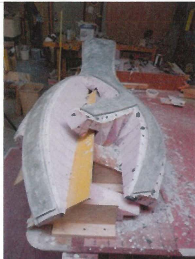
3/8" plaster shell with clay fence removed.
