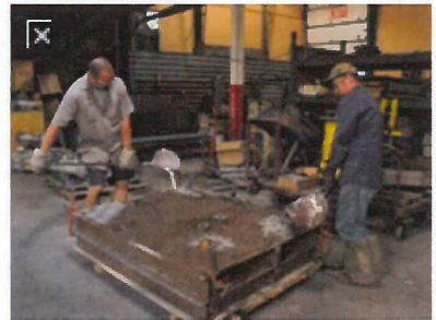
Pouring the melted aluminum.
