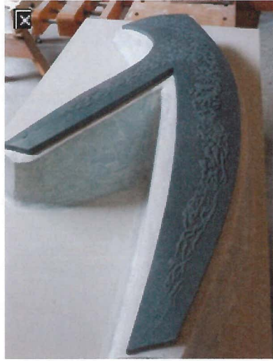
Plaster patterns on follow boards.
