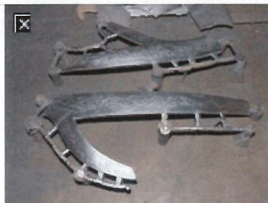
Rough castings with vents and gates.
