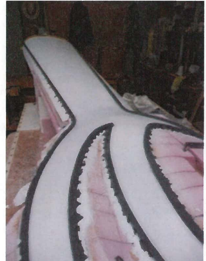
Styrofoam is coated with a smooth coat of plaster and a clay fence 3/8" thick applied to define the outside shape of the sculpture.
