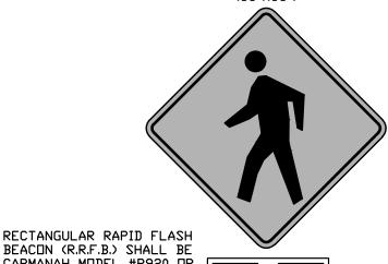
BEACON (R.R.F.B.) SHALL BE CARMANAH MODEL #R920 OR EQUAL. (2 PER EACH DOUBLE-SIDED SIGN)
