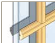
7/8" Simulated-Divided-Light Without Spacer
