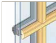
7/8" Simulated-Divided-Light with Spacer
