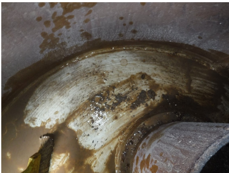
57) Coating failures on the bottom of the riser.
