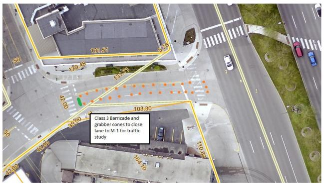
**Figure 2: Temporary Barricade Placement**
