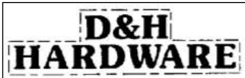
Figure 1: Example of how a sign area is determined by drawing a polygon (indicated by the dashed line) around all type and markings associated with the sign.
