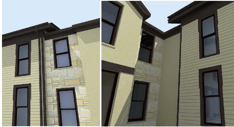
FIGURE 5-6: "HYPHEN" CONNECTION AT HISTORIC STRUCTURE
