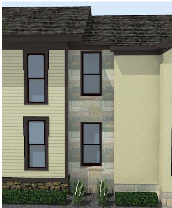
FIGURE 7: LOWER ROOF CONNECTION AT HISTORIC STRUCTURE
