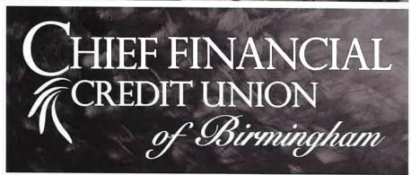
) 79.25" x 33" routed aluminum panel. inel to be stood off from wall with LED backlighting to create halo effect. hite aluminum panel to be mounted to wall for light reflectivity.
