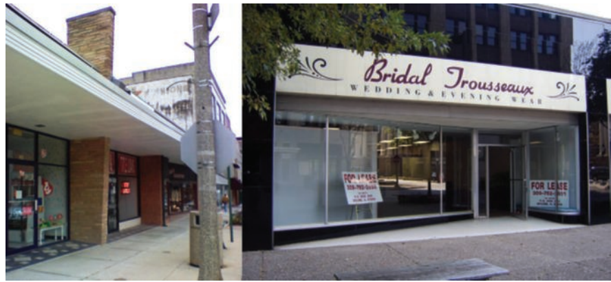
Figure 2: Other postwar design components that occurred parallel with, or as part of open-front designs were asymmetrical and angled fronts. On the left in Freeport, Illinois, angled rustic-stone pylons combine with a deep overhang to shield the open storefront windows from glare. On the right, in Moline, Illinois, is an example of a common postwar open storefront plan, shown here with structural glass surrounding large plate glass display windows that asymmetrically angle into the entrance.
