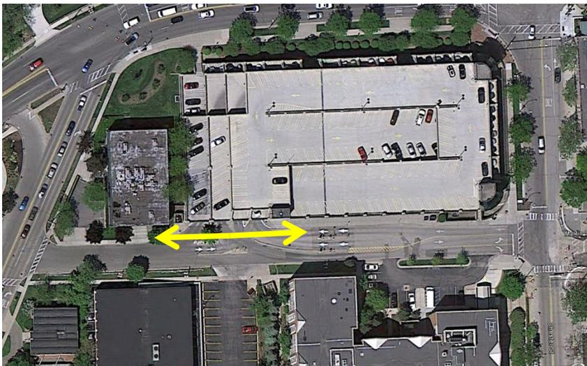
It is recommended that high visibility crosswalks markings be painted across the parking garage entrance as well as providing a sidewalk across the “pork chop” diverter island located between the parking garage entrances.
