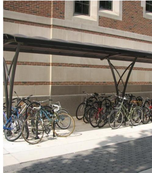
Definition of a Bicycle Parking Space- A bicycle parking space is an area two feet by six feet or the area occupied by a bicycle when using a bicycle parking device as designed.
