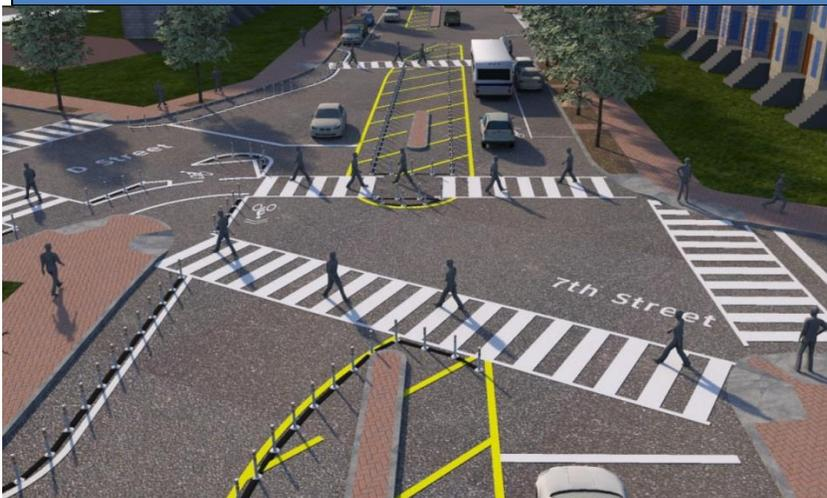
This graphic provides an example of how flexible posts and temporary curbs can be used to pilot changes to roadway configurations.
