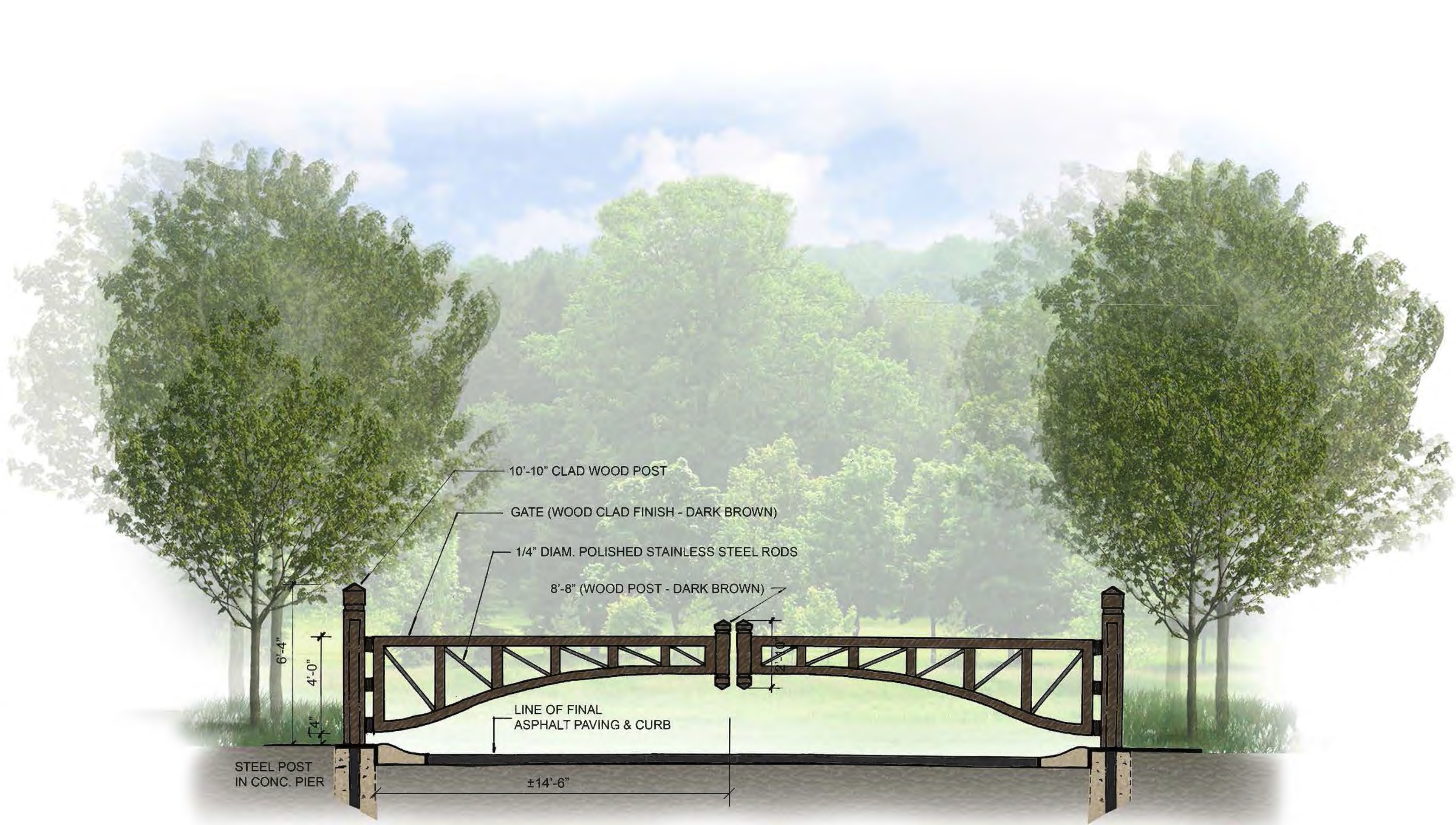
ELEVATION - MOTORIZED GATE
