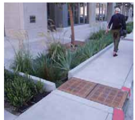
In addition, they can be designed to filter stormwater run-off from street. If there is a raised curb around the parkway as in this example, the access strip next to the curb must be wider than 18".
