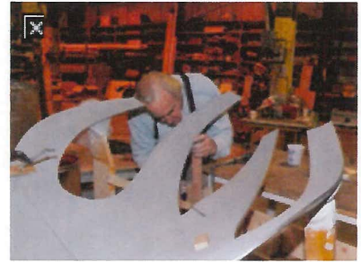
Cast aluminum section being adjusted on jig.
