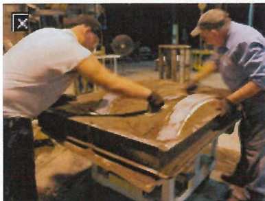
Packing the sand around the pattern in a steel frame.
