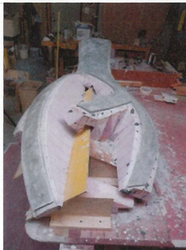
3/8" plaster shell with clay fence removed.
