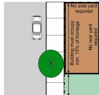
Form-Based Code Building Placement Regulations
