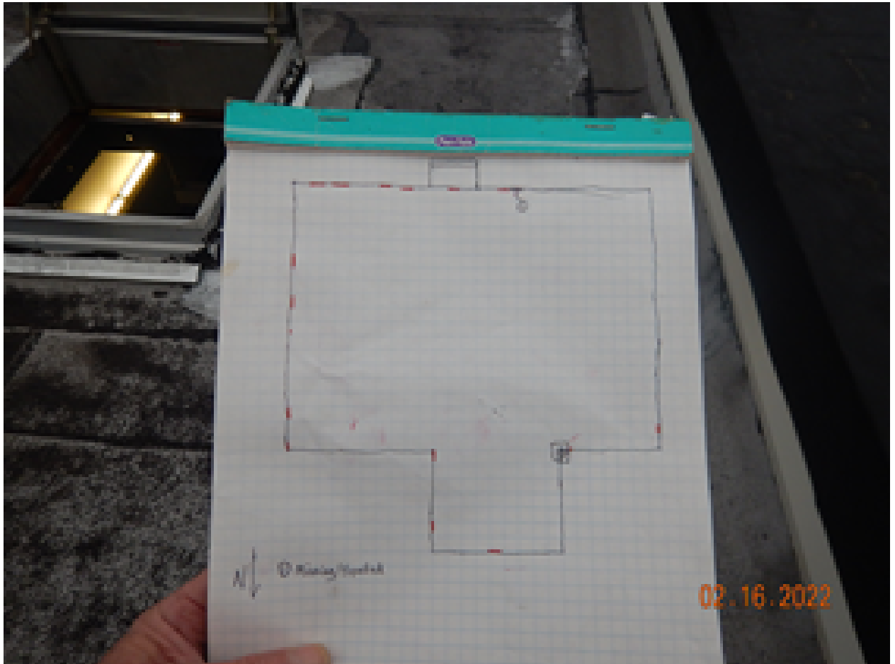
23. View of hand skitch roof plan showing approximate locations of potential cracked/spalled bullnose identified during review.
