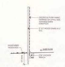
Typ. Silt Fence Detail
