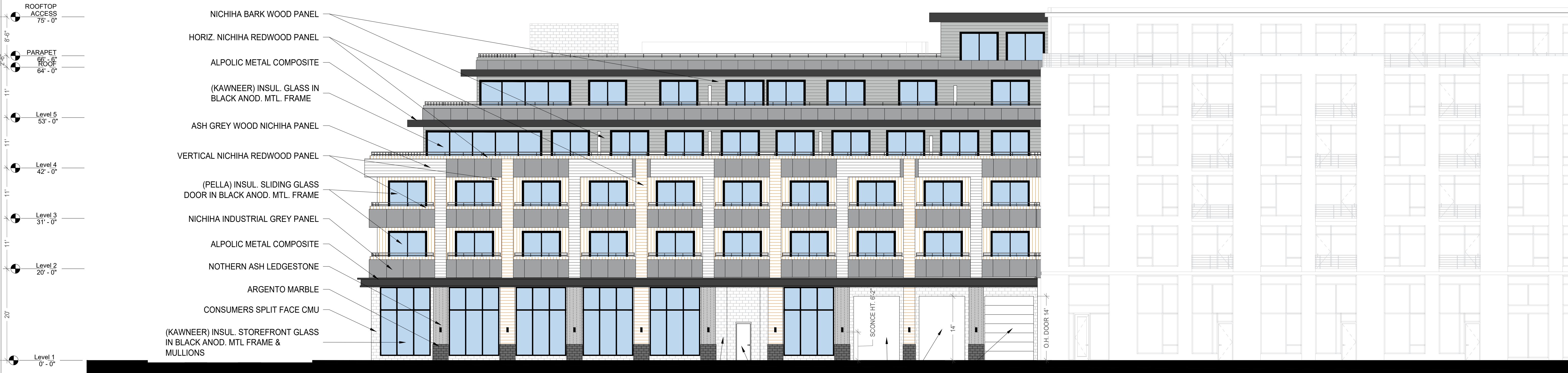
NORTH ELEVATION - HAYNES ST SCALE: 3/32" = 1'-0"
