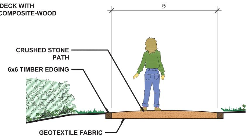
**CRUSHED STONE PATH - SECTION VIEW**
