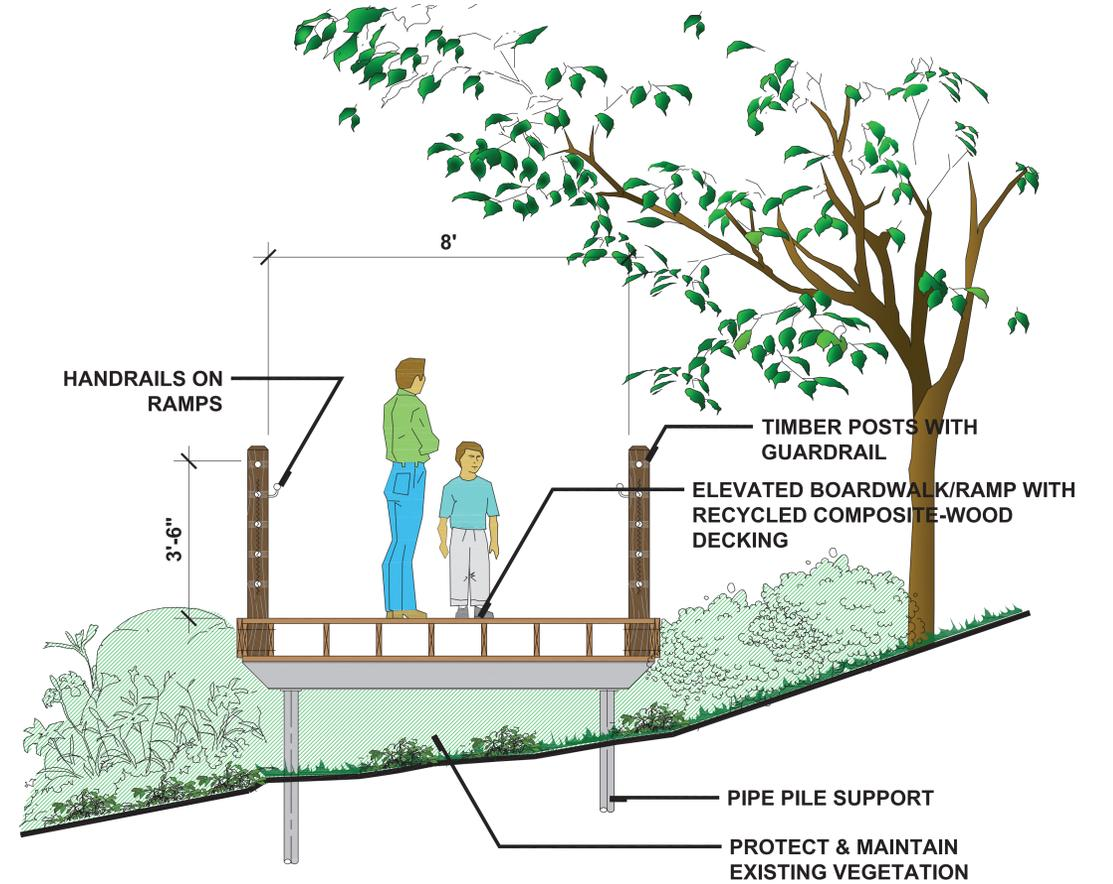
**ELEVATED BOARDWALKS AND RAMPS - SECTION VIEW**
