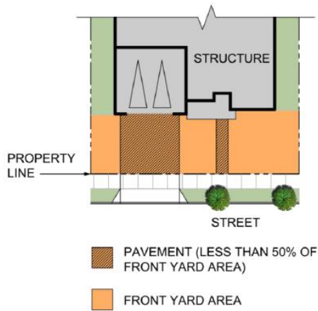
Figure B. Pavement/Hardscape Requirement
