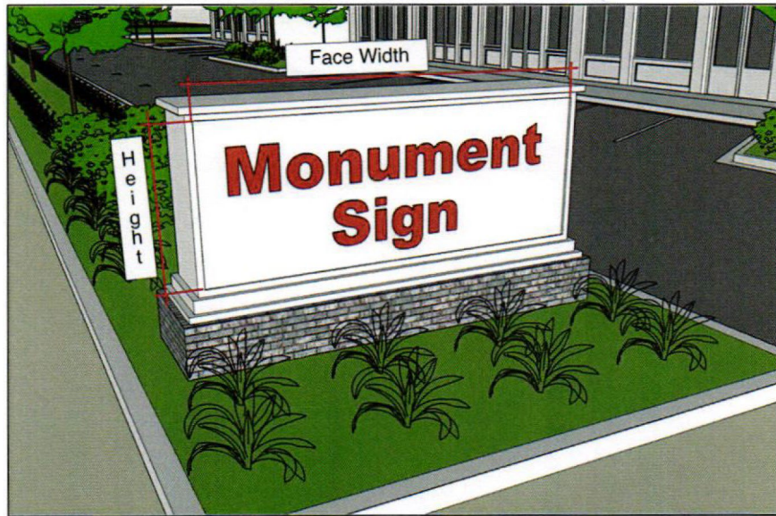
Figure 18: Sign Area Measurement
