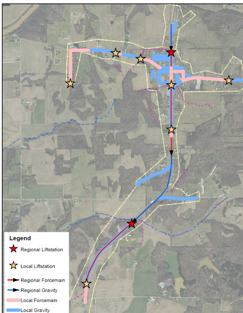
Figure 4-4. Option 1C - Haysville Sewer Network
