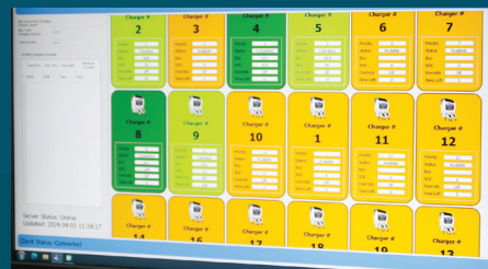
Computerized charging allows vehicle technicians to monitor the battery health and state of charge for each electric bus.
