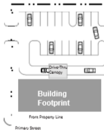
Figure 5.13 (2). Recommended Drive-Through Facility Layout.
