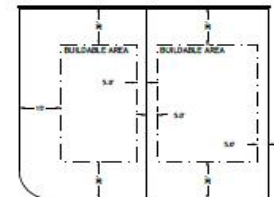
TYPICAL SINGLE FAMILY SETBACK DETAIL NOT TO SCALE
