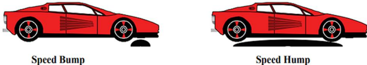
FIGURE 1 Schematic differences between a speed bump and speed hump.
