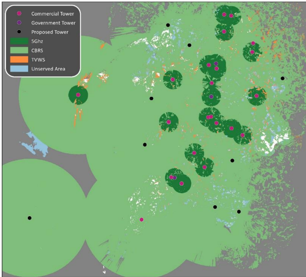
Figure 22: Total Coverage Using Existing and New Towers
