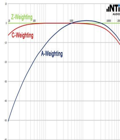
Figure AS The “A” weighting network; low frequency sound energy is rolled off
